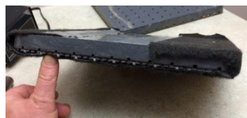
Good clamping of a geocomposite
