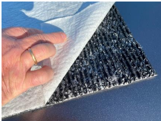
Fig 1—Polypropylene Geomat with geotextile
