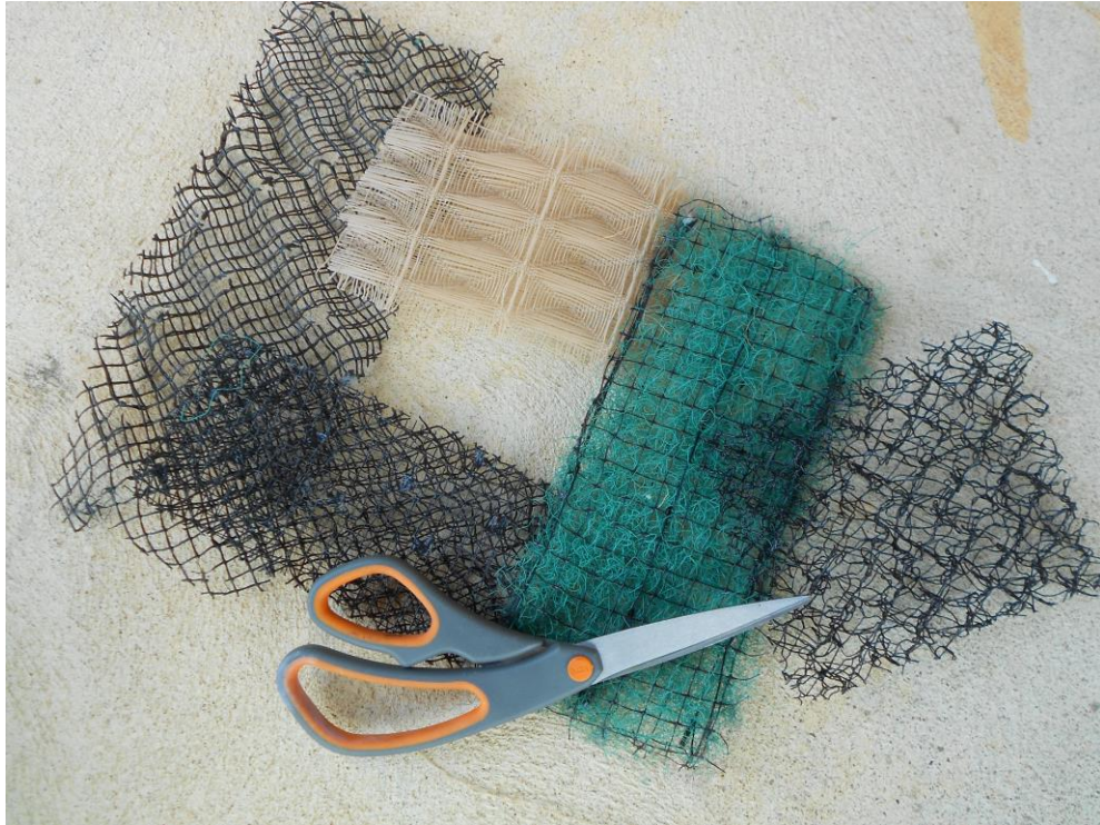
Figure 1 - Array of various turf reinforcement mats (TRMs).
