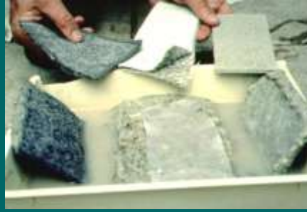
As-Received (Upper Samples) vs. Fully Hydrated (Lower Samples)
