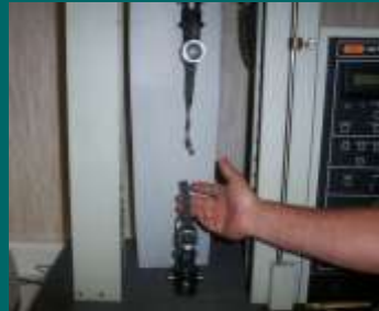
ASTM D882 Narrow (25 mm wide) Strip Tensile Test
