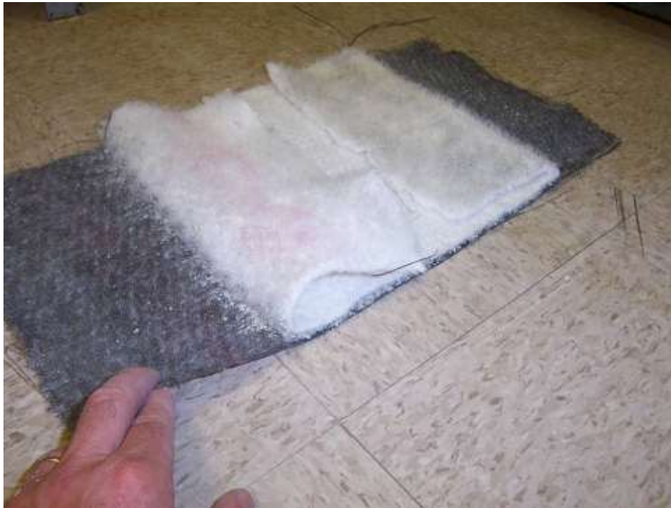
Figure 6. Preparation of the 1 ft (300 mm) wide by 2 ft (600 mm) long GCL specimen. 6 in. (150 mm) of each end is delaminated by hand to facilitate wrap around attachment.
