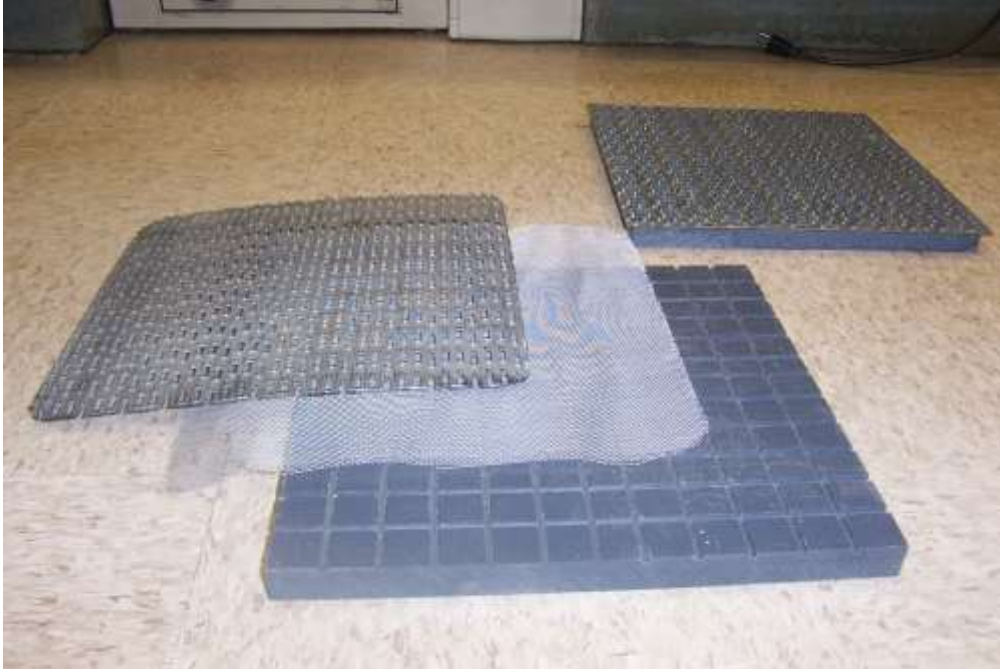
Figure 5. Internal clamps/grips assembled in background and apart in foreground.
