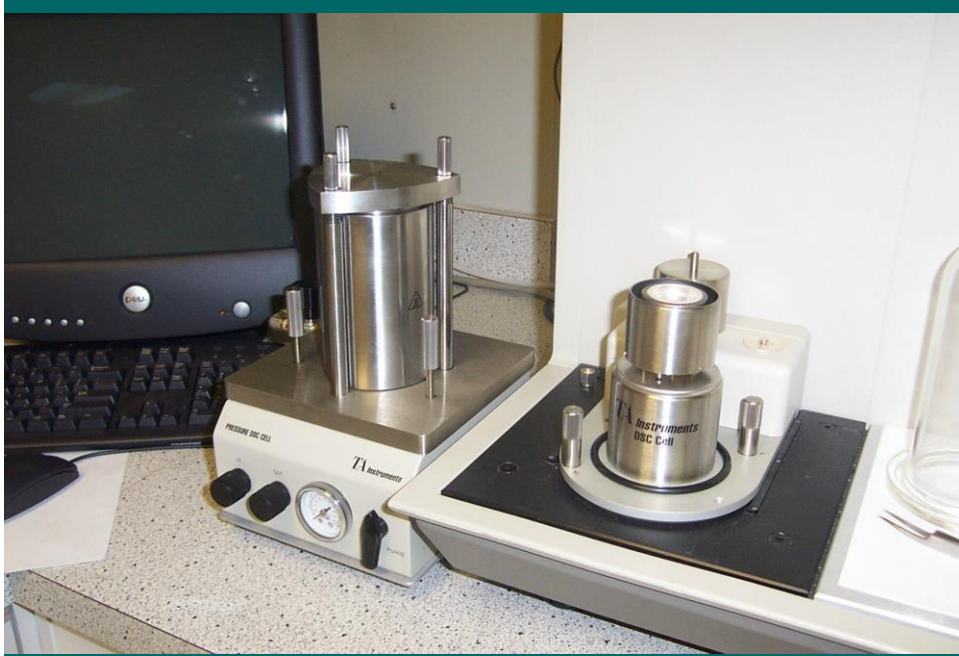
High Pressure (Left) and Standard (Right) Cells for Measuring OIT
