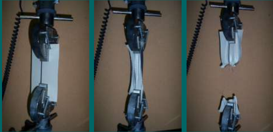
ASTM D751 – Grab Tensile Test in Progress for Reinforced
