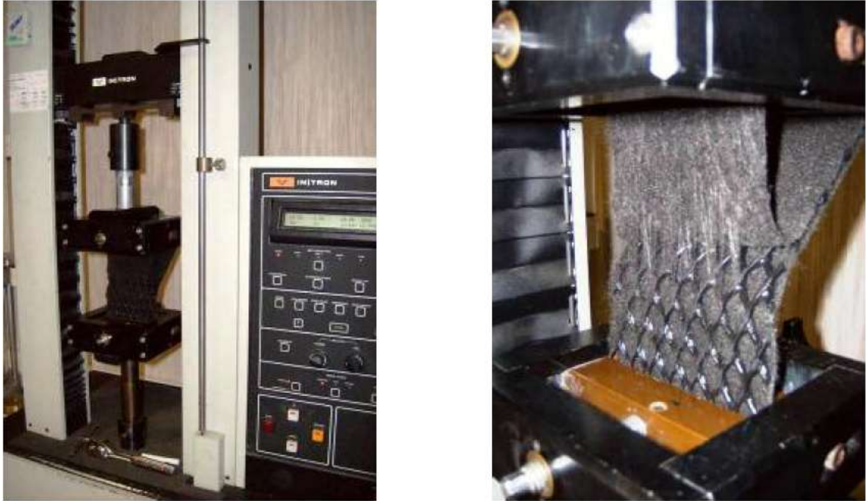
Figure 2. Peel testing of a drainage composite per ASTM D7005.
