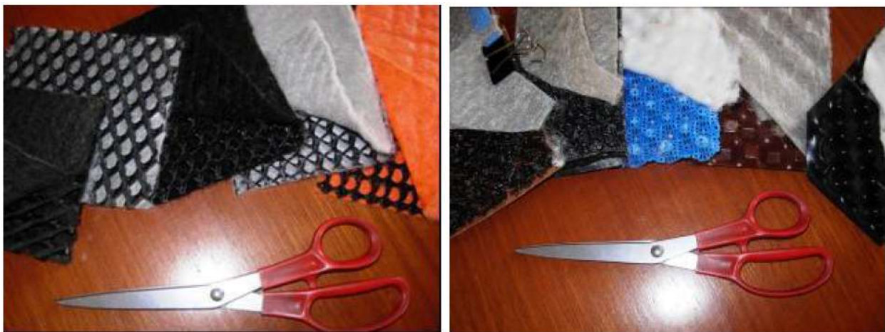
(a) Geonet composite drains
