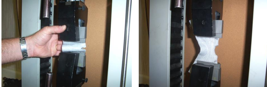
D4533 - Trapezoidal Tear Strength (Measures the Maximum Value)
