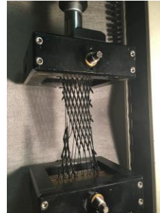
(c) test at failure
