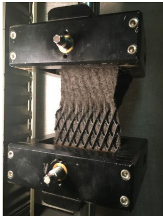
Ply Adhesion Test (ASTM D7005) at Midtest and Failure
