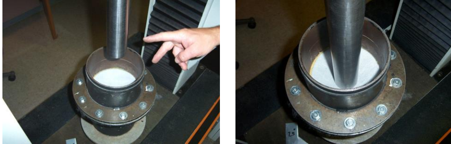
D6241 - Puncture (CBR) Strength (Measures Strength at Rupture and Accompanying Deformation)
