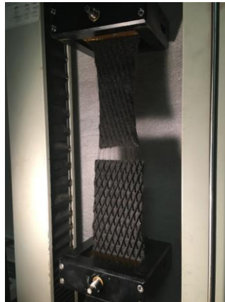
Ply Adhesion Test (ASTM D7005) at Midtest and Failure
