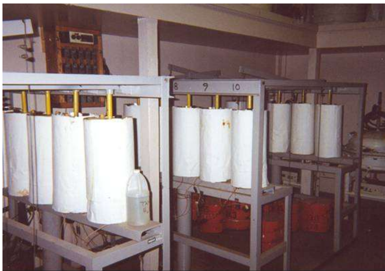
Figure 4 – Devices to incubate coupons under several degradation mechanisms (ref. Koerner, 2012).
