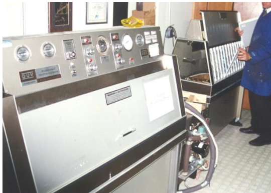
(b) Outside and inside of a fluorescent ultraviolet device Figure 3 – Different ultraviolet incubation devices.
