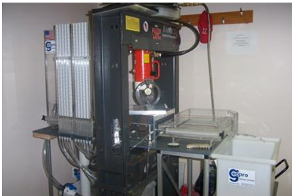
Figure 5. In-plane flow rate testing device per ASTM D4716, (comp., GSI).
