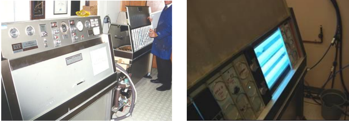
(b) UV Fluorescent Device and Sample Incubation Holders per ASTM D7238
