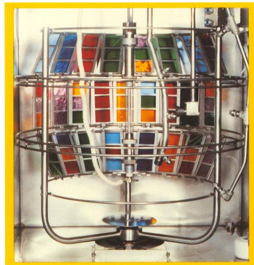
(a) Xenon Arc Device and Sample Incubation Chamber per ASTM D4355
