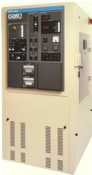
(a) Xenon Arc Device and Sample Incubation Chamber per ASTM D4355
