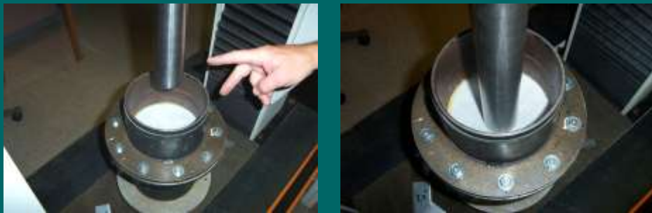
D6241 - Puncture (CBR) Strength (Evaluates Strength at Rupture and Accompanying Deformation)
