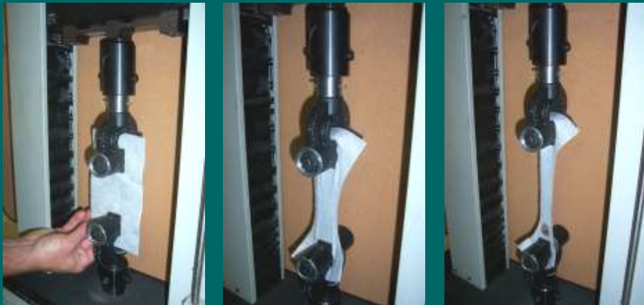
D4632 - Grab Tensile Test (Evaluates Strength and Elongation at Failure)
