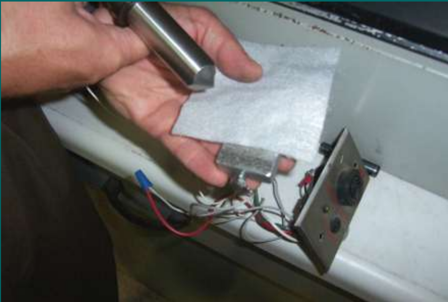
D5494 - Puncture (Pyramid) Strength (Evaluates Strength at Metal Base Plate Contact)
