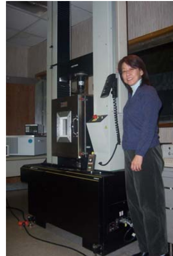
Figure 1 - Grace Hsuan with the CRE donated by the U.S. EPA (Dave Carson). It is equipped with an environmental control chamber, video extensometer and process control creep software. It allows us to accredit ASTM D6992 SIM plus other routine tests.
