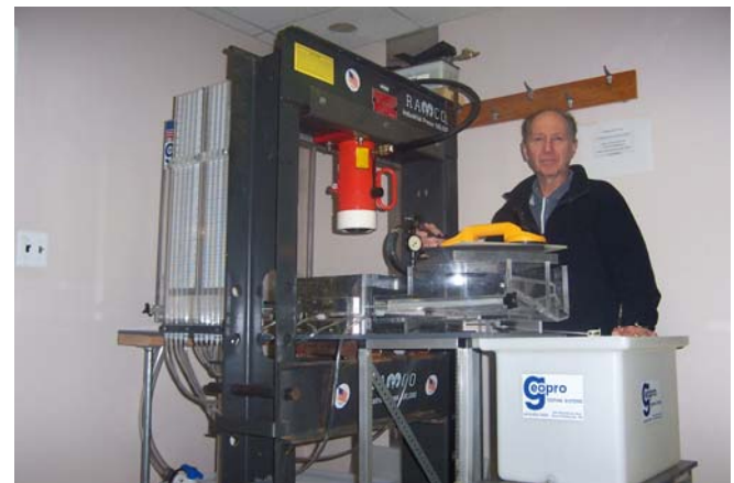
Figure 2 - Bob Koerner with new transmissivity unit donated by Geotechnics (Rich Lacey). It is equipped with a precise machined specimen box which allows for monitoring of head in various locations. This box limits side wall leakage and has nice upstream
