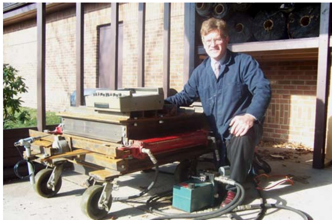
Figure 3 - George Koerner with new pullout unit donated by SGI Testing Services, LLC (Robert Swan and Zehang Yuan). This box replaces one that we were unable to move from Drexel. It is versatile and can run both ASTM D6638 connection strength and ASTM D6706 pullout resistance.
