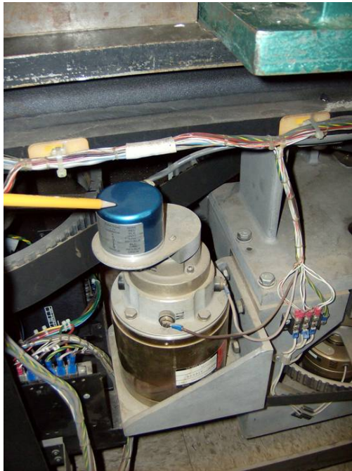
Figure 2. Odeometer or LVDT in the CRE machine for measuring crosshead movement.
