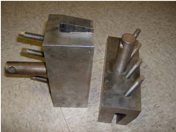
Figure 1. Wedge type grips per ASTM D4595.
