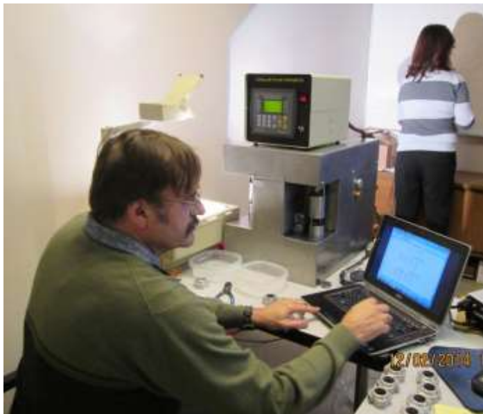
Richard Lacey of TRI operating the Capillary Flow Porometer
