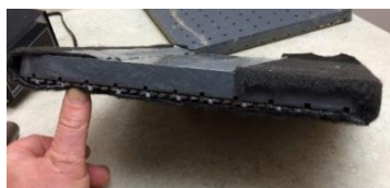
Good clamping of a geocomposite
