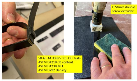
Better extrusion welds, Aquatan SA 20 year old field seams from Onverwacht Dam 1 & 2B
