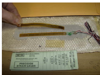
(a) - Photograph of foil strain gauges. Note one is attached to geotextile.
