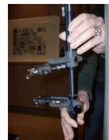
(a) - Photograph of clip-on extensometer (b) - Photograph of cable "roller style" extensometer
