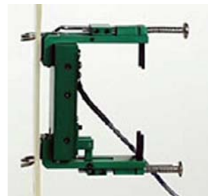
(a) - Photograph of clip-on extensometer (b) - Photograph of cable "roller style" extensometer
