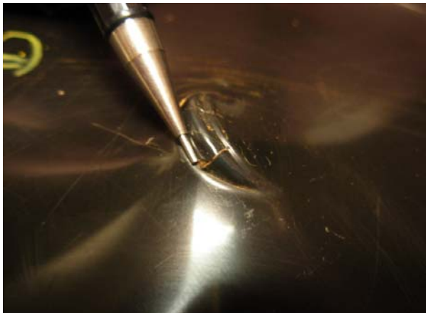
(b) Deformation from 38 mm cone heights; Vessels No. 3 and 4
