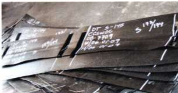
(a) Test samples with destructive test specimens removed
