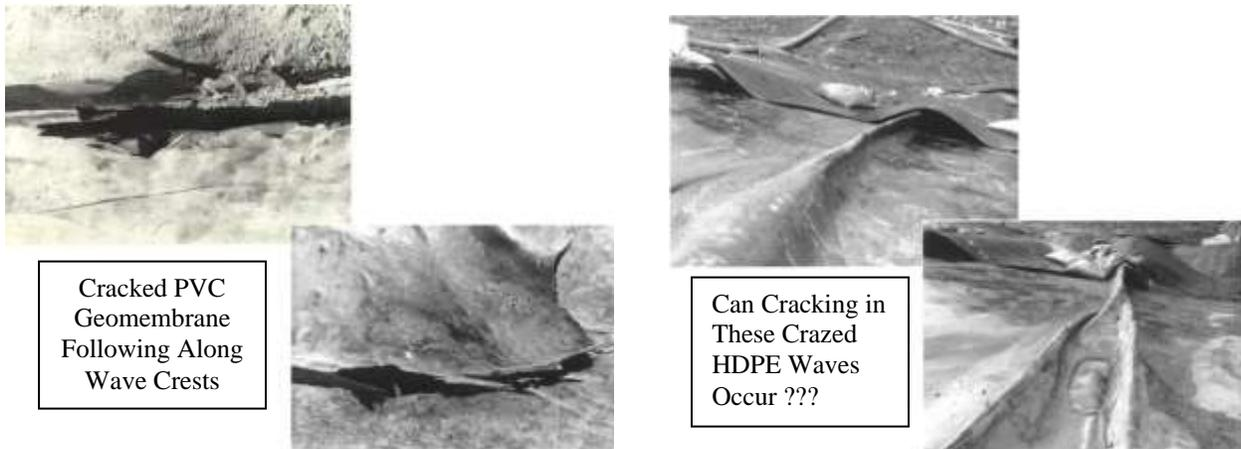
(a) Cracking of PVC geomembranes
