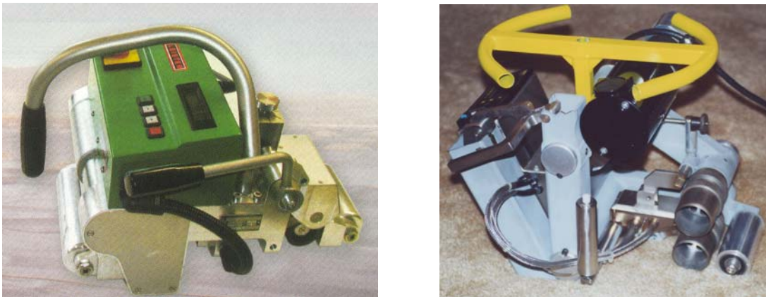
Figure 4 – Two Variations of Automatic Wedge Welding Devices (compliments of Leister Inc. and Fred Struve)
