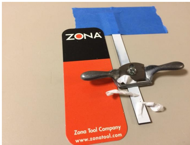
Figure 6. Small plane removal of white layer from multilayered geomembrane. (GSI photo)
