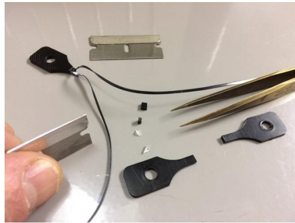
Figure 7. Planar separation of layers after test specimen straining. (GSI photo)
