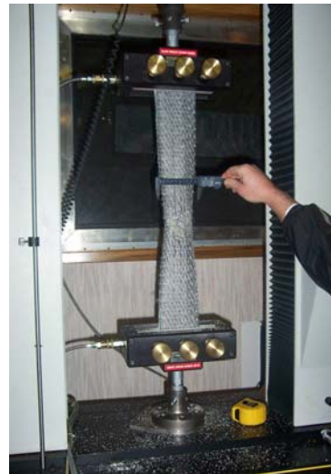
(b) Woven/Nonwoven Reinforced GCL per ASTM D6768 (Confidential site in Table 1) [150 mm (L) × 100 mm (W); aspect ratio = 5.0]
