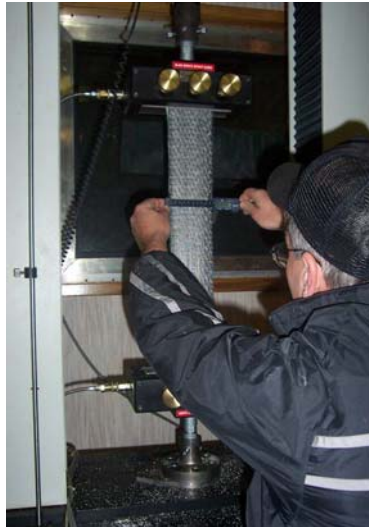
(b) Woven/Nonwoven Reinforced GCL per ASTM D6768 (Confidential site in Table 1) [150 mm (L) × 100 mm (W); aspect ratio = 5.0]
